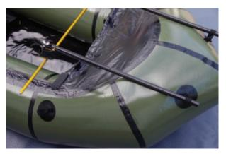
6. Next, insert the crossbar in the rear loops. The width is adjusted by sliding the rod holders laterally on the aluminium crossbar.
