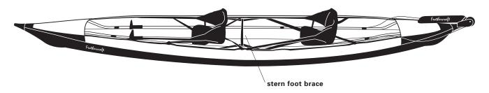
When using the rudder, run the cables under the deck webbing, and through the gunwale velcro closures to the bow foot braces.
