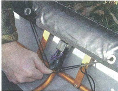
Figure 8 Hook string loops to the frame
