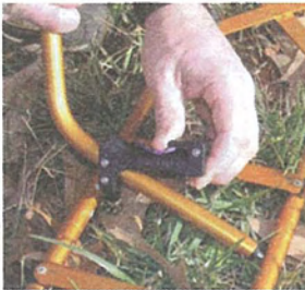
Figure 3 Installing cross rib
